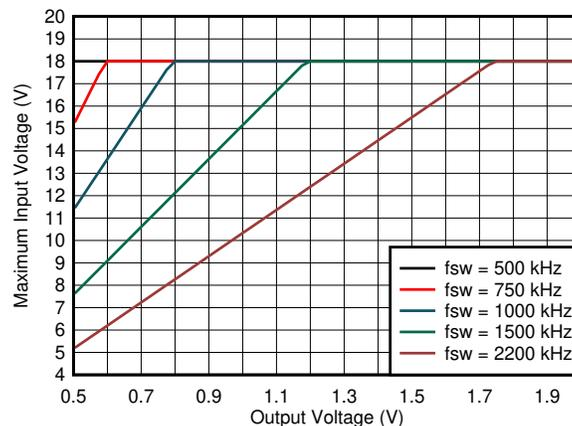
Figure 8-2. Maximum Input Voltage vs Output Voltage
