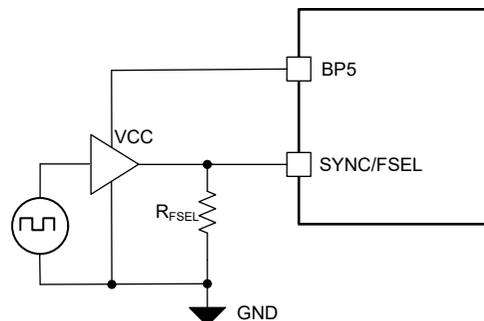
Figure 7-4. Interfacing the SYNC/FSEL Pin with a Buffer
