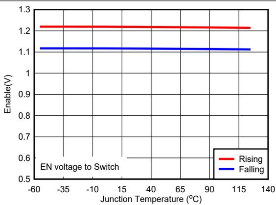
Figure 6-5. Enable Voltage
