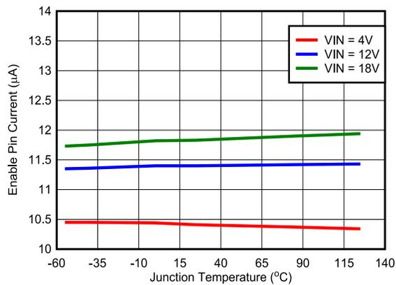
Figure 6-11. Enable Pin Current at Different VIN
