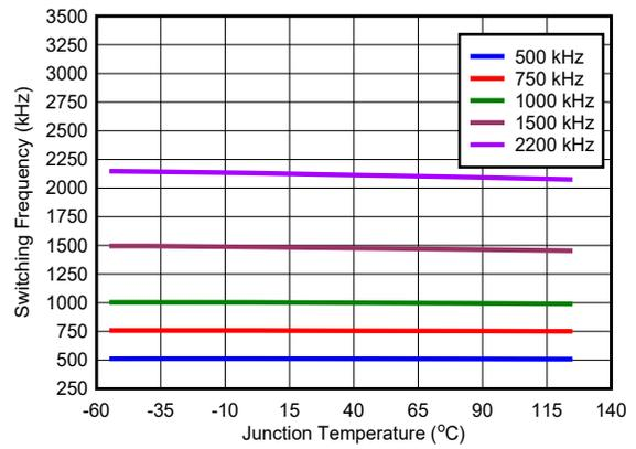
Figure 6-16. Switching Frequency vs Temperature
