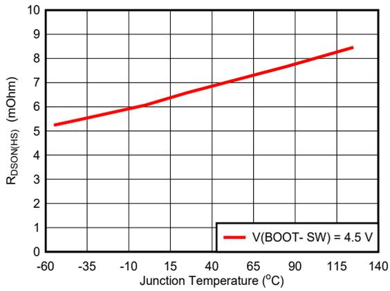
Figure 6-1. High-Side FET Rd<sub>ON</sub>
