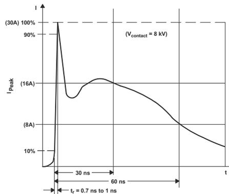
Figure 9-5. Typical Current Waveform Of IEC61000-4-2 ESD Generator
