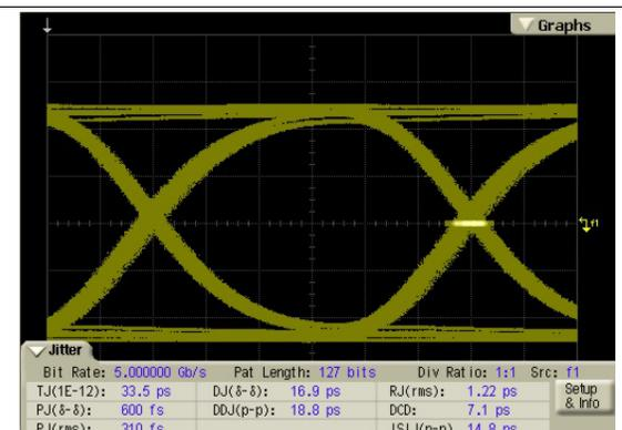
Figure 7. 5-Gbps Output with 20 Inch Input Trace and 13-dB EQ Setting
