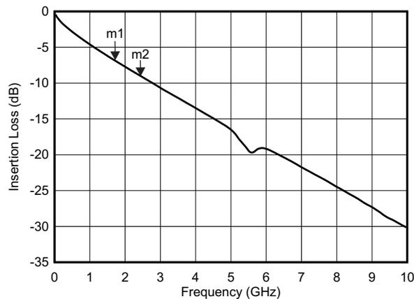
$$m1 \text{ frequency} = 1.876 \text{ GHz} \qquad I_L = -7.346$$
