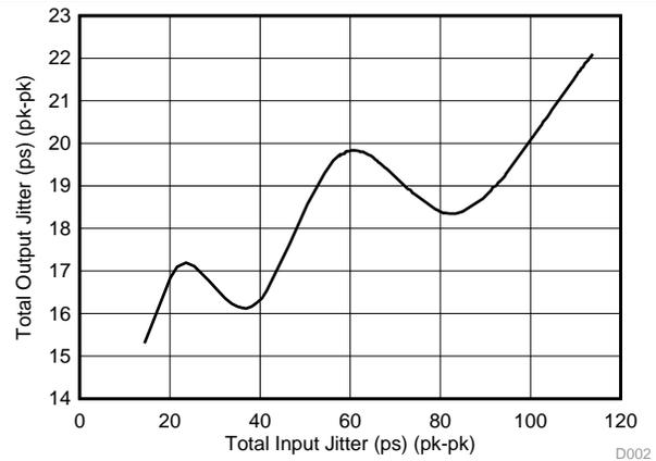
Figure 3. Jitter Performance with Optimal EQ Settings
