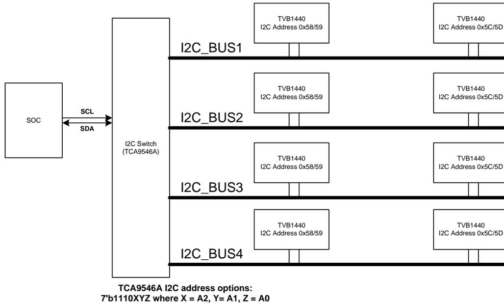
**Figure 11. Example I2C Switch Implementation****9.1.1.2.5 Receiver Equalization Setting**
