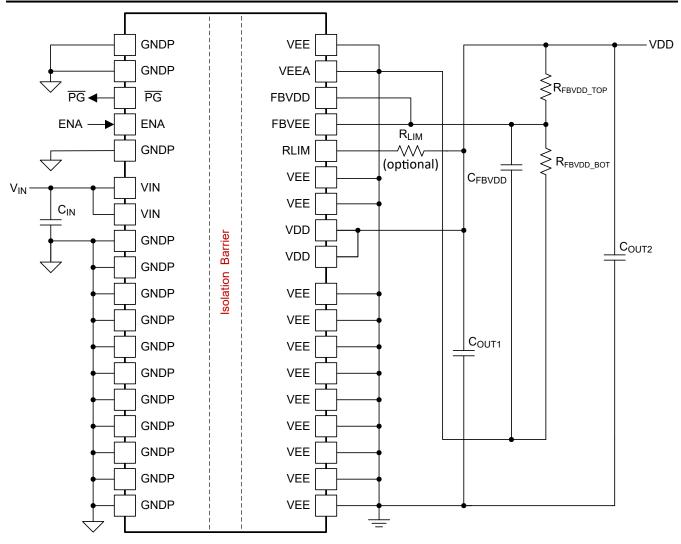
図 8-2. Single Adjustable Output Configuration
