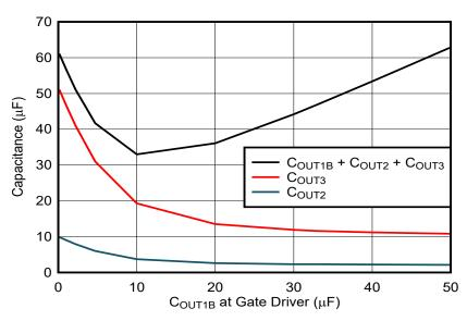
図 8-5. Output Capacitance Variation with Cout1B selection
