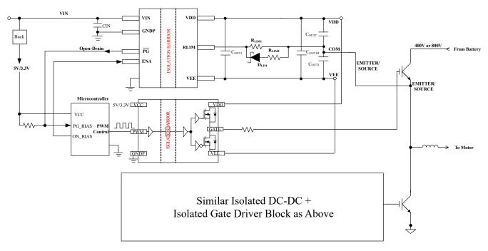
図 8-11. Dual Output System Configuration
