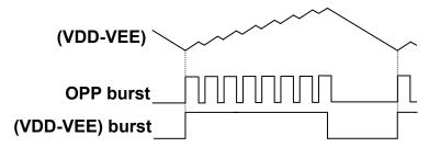
図 7-4. Diagram of Over-Power-Protection with Baby Burst
