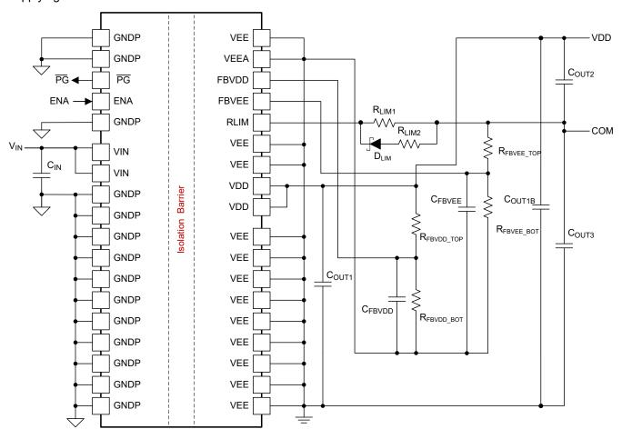
図 8-1. Dual Adjustable Output Configuration
