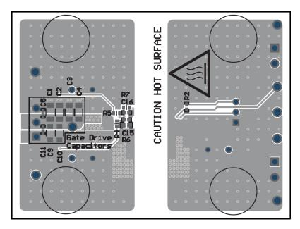
図 8-24. UCC14341-Q1EVM, PCB Bottom Layer, Assembly (Mirrored View)
