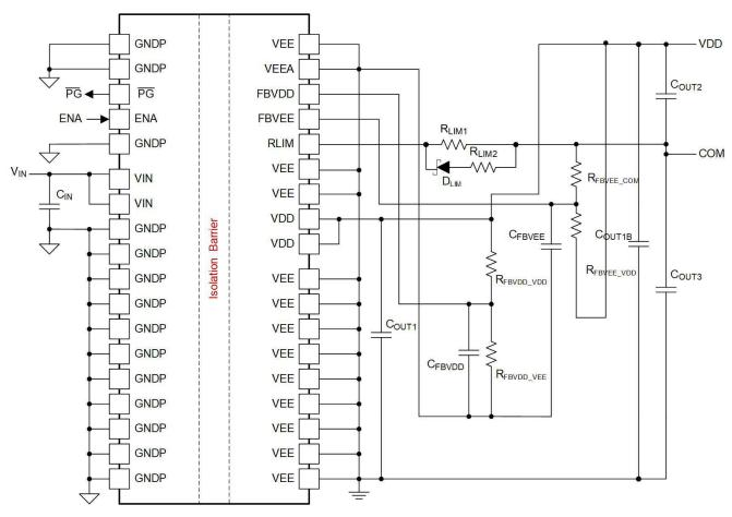
$\boxtimes$  8-10. Dual output application schematic configured for  $V_{COM\_VEE}$  regulation < 2.5V
