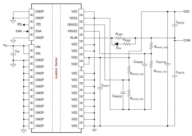
$\boxtimes$  8-8. Dual output application schematic configured for  $V_{COM\_VEE}$  regulation > 2.5V
