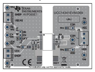
図 8-21. UCC14341-Q1EVM, PCB Top Layer, Assembly
