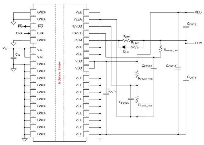
$\boxtimes$  8-9. Dual output application schematic configured for  $V_{COM\_VEE}$  regulation = 2.5V
