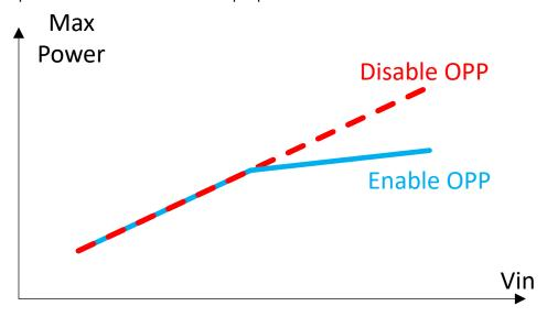
☑ 7-8. Maximum Output Power Under Different Input Voltage Condition
