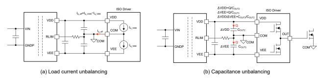
図 8-7. Source of Voltage Unbalancing
