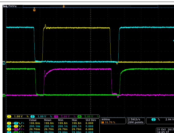
Figure 9-6. Zoomed-In bench-test waveform
