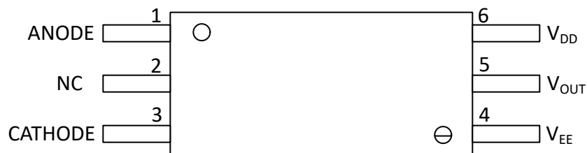
図 5-1. UCC23113 DWY Package SOIC-6 Top View
