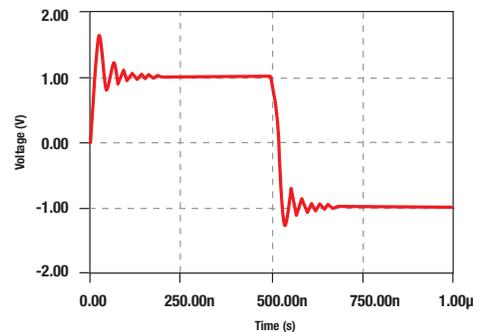
Step response of amplifier with limited capacitive load drive: non-ideal behavior – ringing effect, slow recovery
