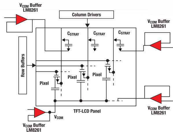
*Displays with larger screens and those that are touch-based often require more than one  $V_{COM}$  buffer.*
