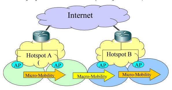
As the diagram illustrates, the hierarchical nature of IP network topology results in two types of mobility:
