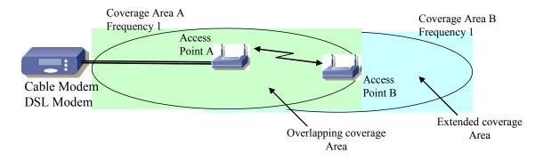
Access point B is a repeater (mesh element) to access point A, which connects to the Internet. Access point A functions as a router to access point B. Access point A must maintain a routing list for all clients in the home network while access point B only must maintain a routing list of attached clients. For example, B may be a simple bridge or a more intelligent router. Clearly, the
