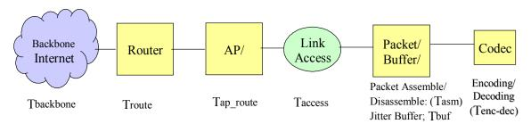
Because delay in the PSTN backbone network is beyond the control of mobile device manufacturers, the following table illustrates a residual delay budget for the backbone network (Tbackbone) using short duration G.711 and G.726 VoIP packet structures. The data for this table is taken from measurements that were performed on TI/Telogy VoIP software implementations and from worst case delays in TI's extensive wireless enterprise network.
