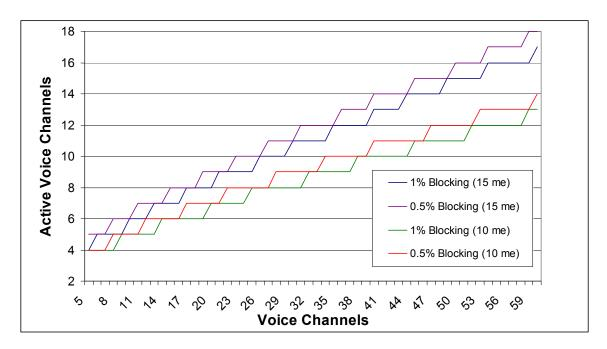
As the pool of attached phone lines increases, efficiency, in terms of fewer blocked calls, and over-subscription also will increase. This should not be surprising because the efficiency of all systems that use statistical multiplexing improves as the number of channel resources increases at the multiplexer. The concentration level moves from around 2:1 at 10 subscriber phone lines to more than 3:1 at 60 user phone lines.
