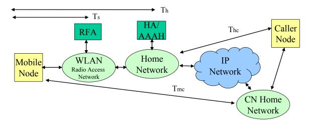
When both caller and the mobile node are in the home network (i.e. when the switching occurs within one's own voice network), the PBX function is present. In this case, the VoIP call is routed through a self-contained enterprise network and no Internet domain resources are required.
