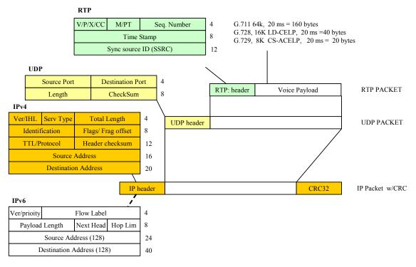
Clearly VoIP has an overhead issue that is compounded when high levels of voice compression are deployed in conjunction with voice packets of short duration. The tradeoff between overhead and packet duration is shown in the following table. Other issues affecting VoIP network capacity planning, such as delay, jitter and packet duration, are discussed later in this white paper.
