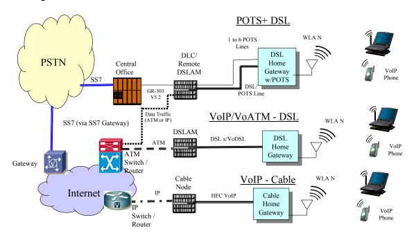
Residential/SOHO customers typically have one or more analog voice circuits which are connected directly to the PSTN through a CLASS 5 switch or through a DLC remote terminal. In many cases, subscribers are served by advanced DLC/DSLAM (DSL access multiplexer) remote terminals that provide a combination of DSL and POTS service on a single line as well as standard POTS voice circuits.
