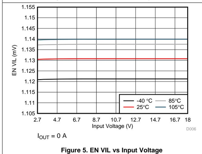
Figure 5. EN VIL vs Input Voltage
