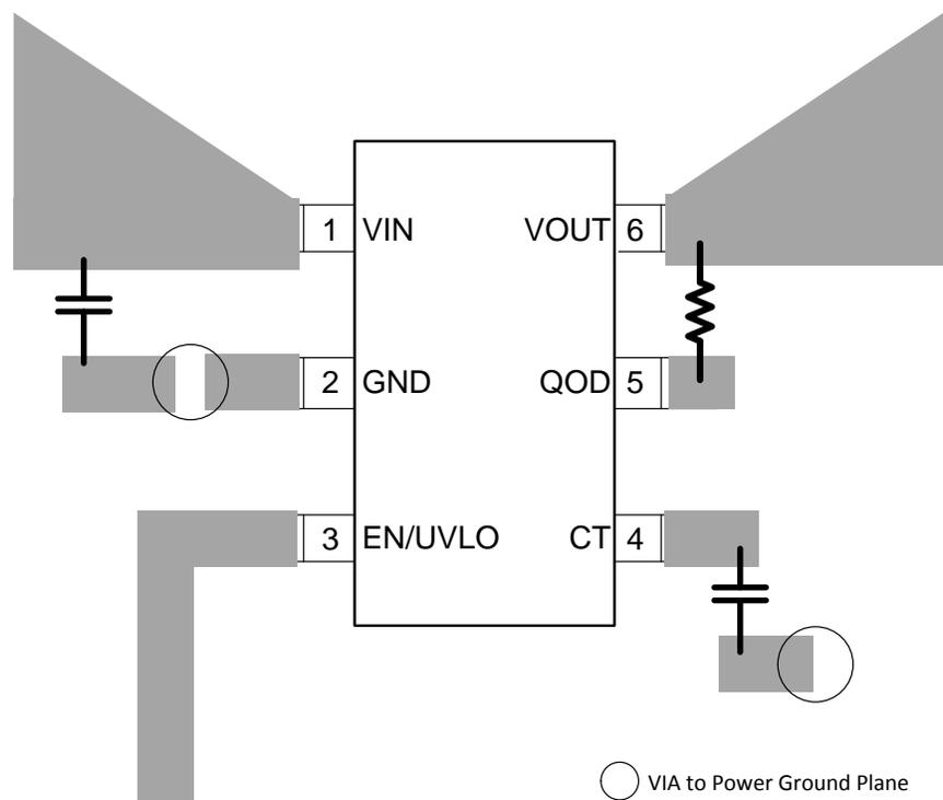
**Figure 34. Recommended Board Layout**
