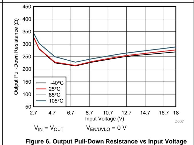
Figure 6. Output Pull-Down Resistance vs Input Voltage
