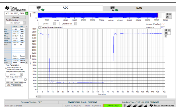
Figure 8-6. 40-MHz, Square-Wave Time Domain for 5-GSPS, Single-Channel Oscilloscope
