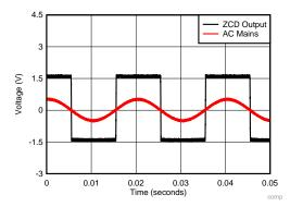
Figure 2. ZCD Output Corresponding to Ideal AC Mains
