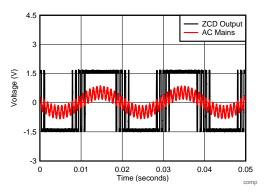
Figure 3. ZCD Output Corresponding to Distorted AC Mains
