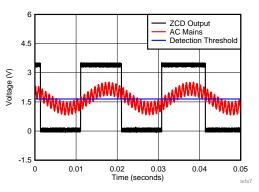
Figure 7. ADS7x28 ZCD Output Corresponding to Distorted AC Mains
