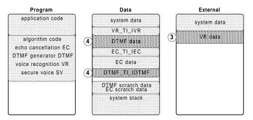
Note that if we want to move an algorithm's data and deactivate it, we must do them in this sequence: move data, call algMoved(), call algDeactivate(). This ensures the algorithms' data pointers are current the next time it is activated.
