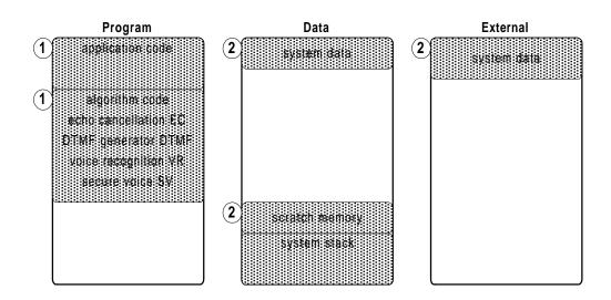
Figure 8. Memory Diagram at Power On
