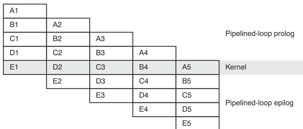
**Figure 4-1. Software-Pipelined Loop**
