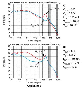
$PSRR_{dB} = 20\log\left[\frac{\Delta V_{IN,pk-pk}}{\Delta V_{OUT,pk-pk}}\right]$
