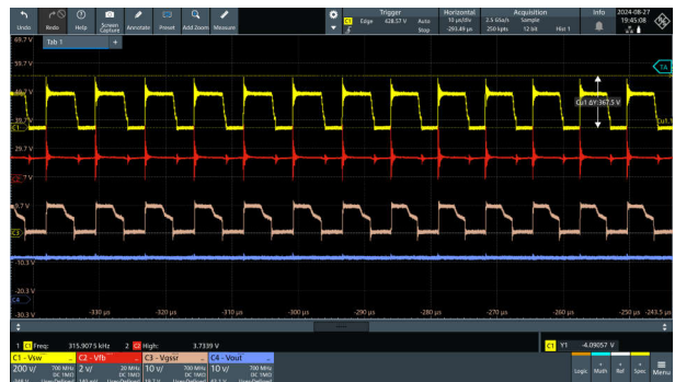
図 3-19. Vin = 115Vac、Vout = 15V
