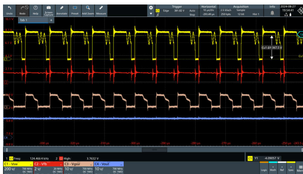
図 3-20. Vin = 230Vac、Vout = 15V
