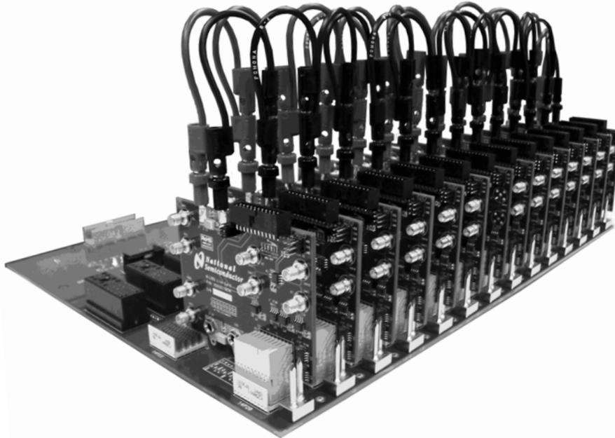
FIGURE 4. 14-Slot ATCA Backplane Fully Loaded with M-LVDS Line Cards
