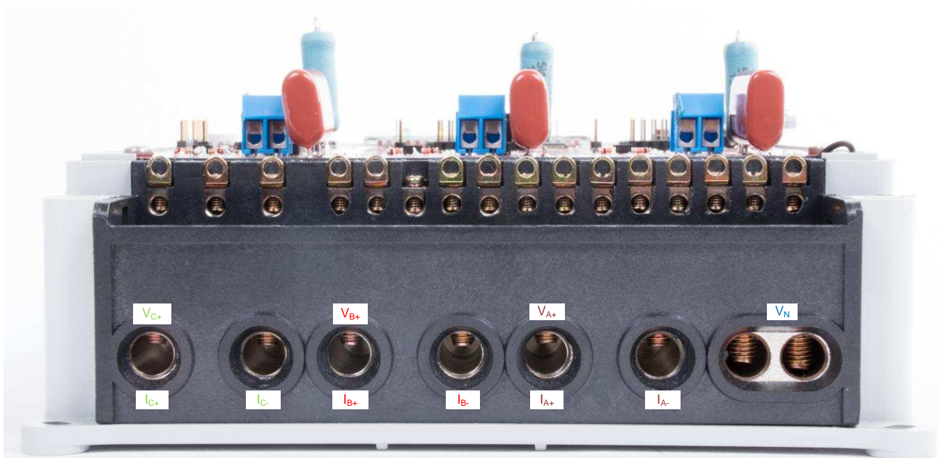
図 21. Front View of EVM With Test Setup Connections
