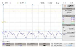
図 3-21. Zoomed-in Ripple Voltage at Load Current of 40 mA
