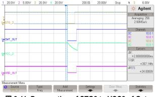
図 3-11. Propagation of STO2 to VCC2 of Gate Driver
