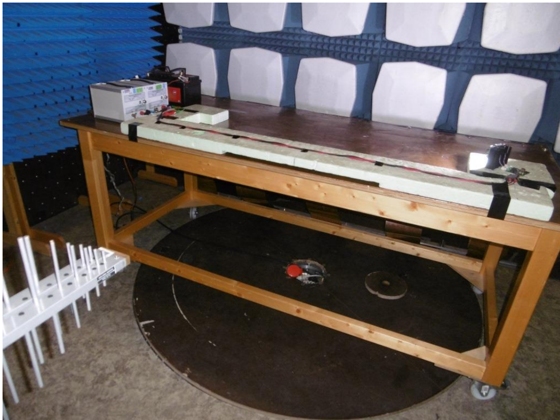
図 26. CISPR 25 Radiated Emissions Setup
