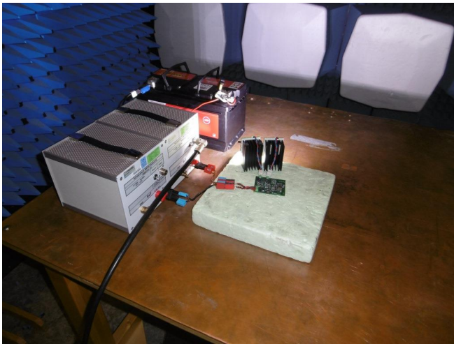
図 24. CISPR 25 Conducted Emissions Setup
