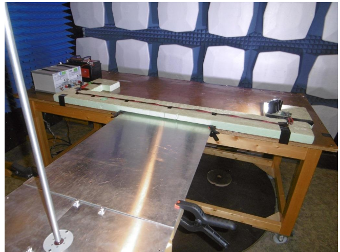
図 25. CISPR 25 Radiated Emissions Setup (Monopole)
