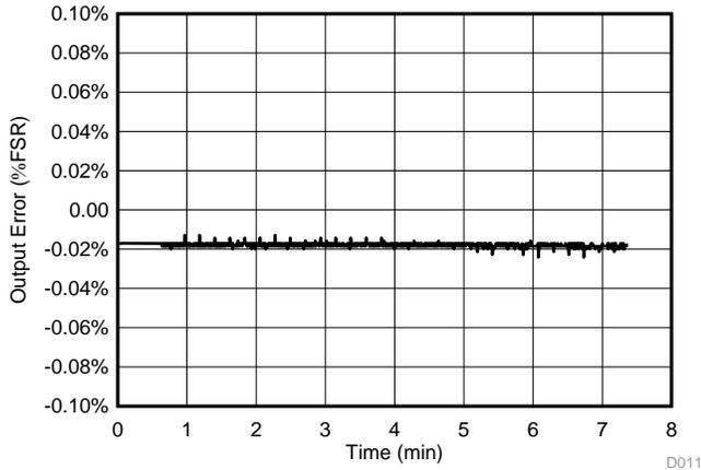
☒ 17. Voltage Output: ±4-kV Electrically Fast Transient
