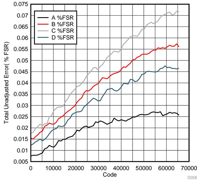
**図 7. Measured Current Output Total Unadjusted Error (%FSR)**
