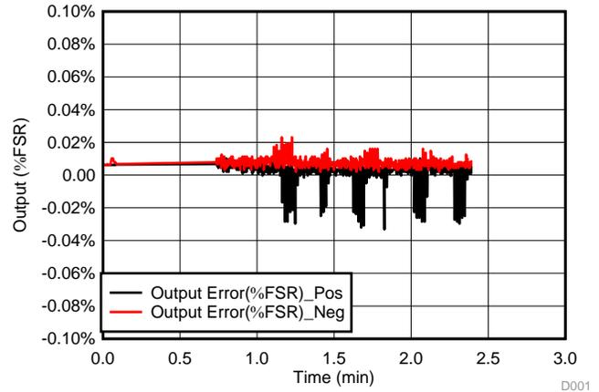
☒ 18. Current Output: ±4-kV Electrically Fast Transient
