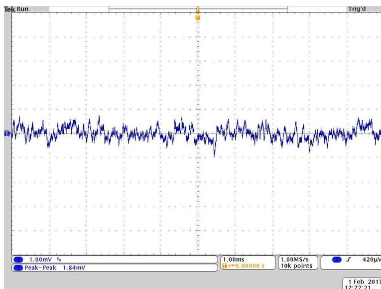
図 10. Measured Output Voltage Ripple
