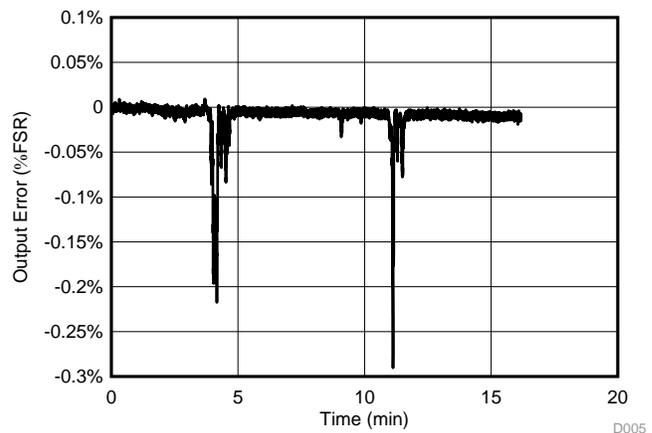
図 16. Current Output: 20-V/m Radiated Immunity
