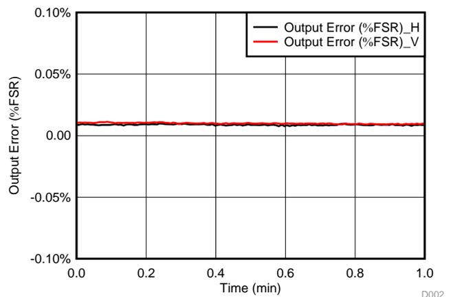
図 14. Current Output:  $\pm 8$ -kV ESD Vertical and Horizontal Coupling Plane Discharge
