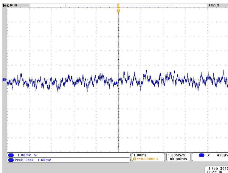
図 9. Measured Output Current Ripple
