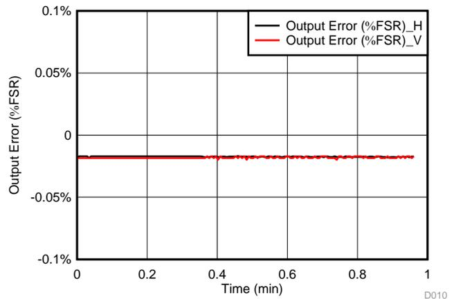
図 12. Voltage Output:  $\pm 8$ -kV ESD Vertical and Horizontal Coupling Plane Discharge
