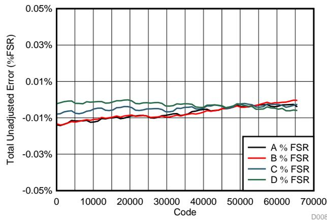
**図 8. Measured Voltage Output Total Unadjusted Error (%FSR)**
