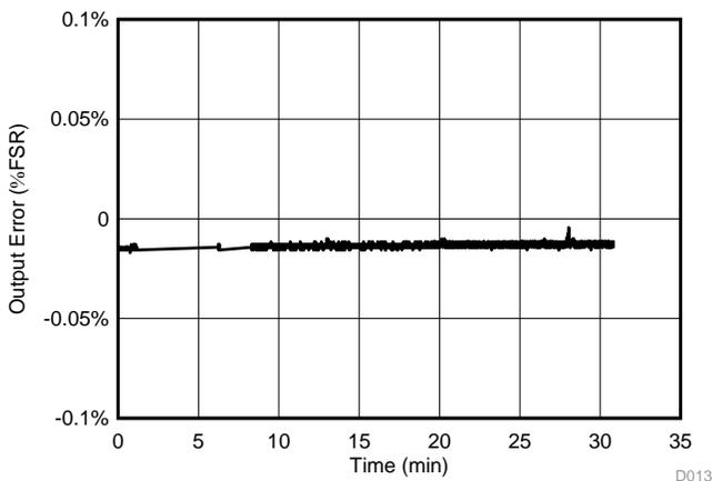
図 15. Voltage Output: 20-V/m Radiated Immunity
