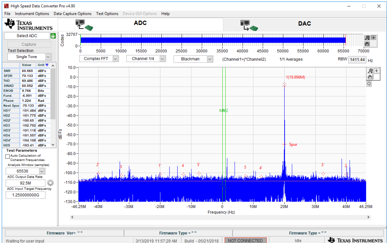
図 35. ADC1 Spectrum - I Data, F_s = 1480 \text{ MHz} , F_{NCO} = 1270 , F_{in} = 1250 \text{ MHz}
