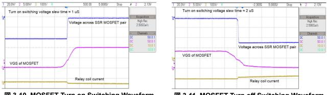
図 3-10. MOSFET Turn on Switching Waveform
