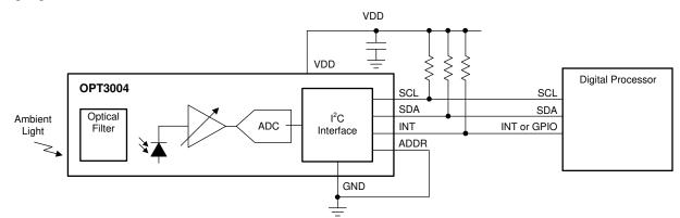
図 2-14. OPT3004 Functional Block Diagram
