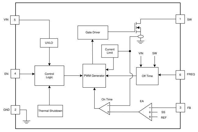
図 2-17. TLV61048 Functional Block Diagram
