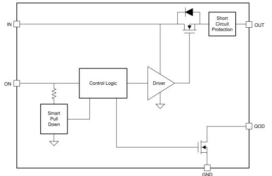
図 2-12. TPS22919 Functional Block Diagram
