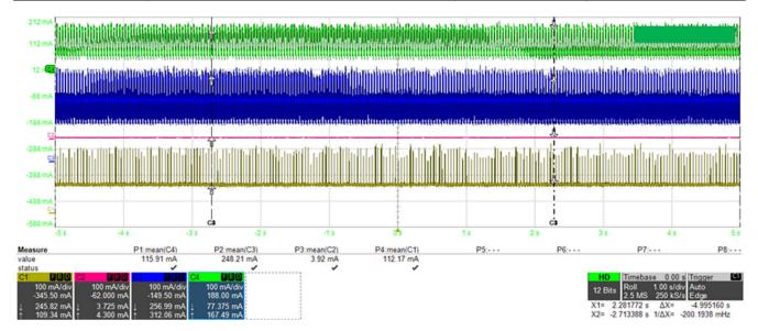
図 3-18. Current Consumption From Each Rail: C1-VOUT1 (3.3 V), C2-1.35 V, C3-1.1 V, C4-1.8 V
