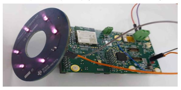
図 3-23. Setup With IR LEDs Connected to the Camera Module
