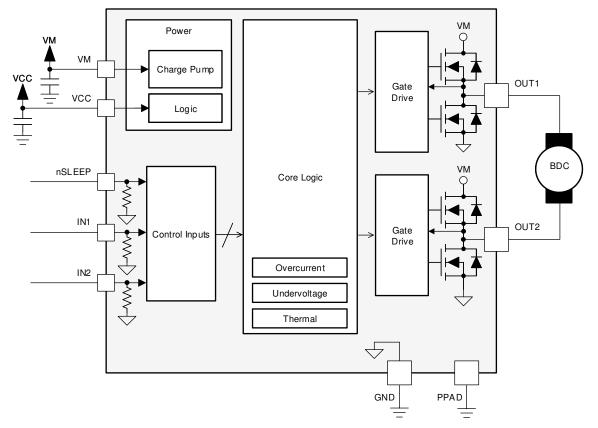
図 2-15. DRV8837C Functional Block Diagram
