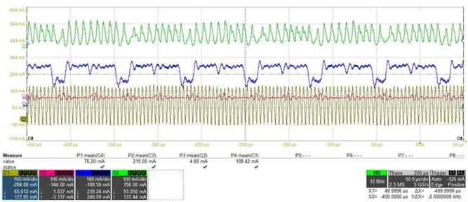
図 3-19. Current Consumption Zoomed in From Each Rail: C1-VOUT1(3.3 V), C2-1.35 V, C3-1.1 V, C4-1.8 V
