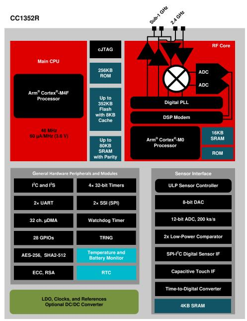
図 2-5. CC1352R Functional Block Diagram
