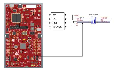
図 3-2. Connections Between CC32xx LaunchPad<sup>™</sup> and Wireless Camera Module (J13 Connector)
