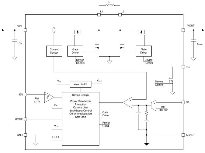
図 2-6. TPS63802 Functional Block Diagram
