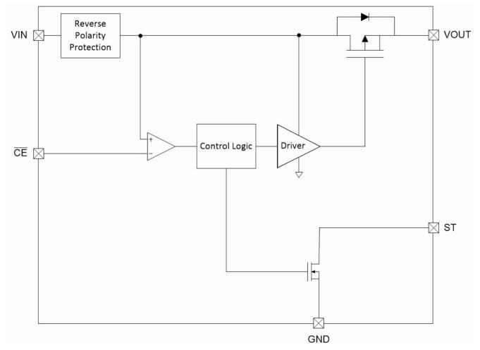
図 2-13. LM66100 Functional Block Diagram
