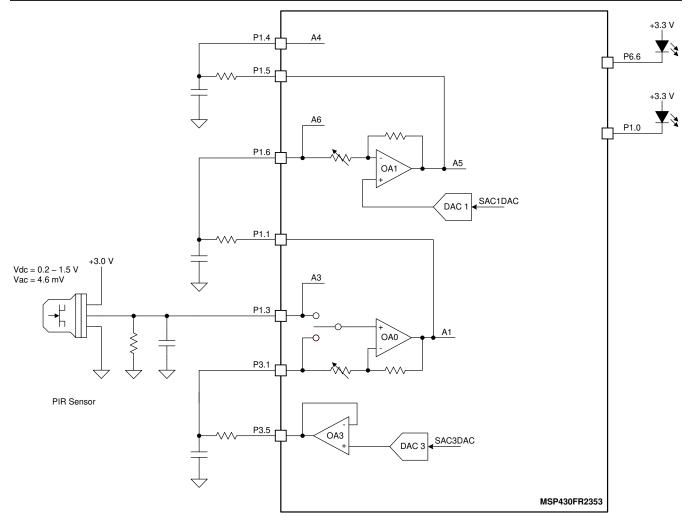
図 2-21. PIR and MSP430<sup>™</sup> Based Motion Detection Design Block Diagram
