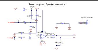
図 2-25. Audio Power Amplifier Circuit in the Design
