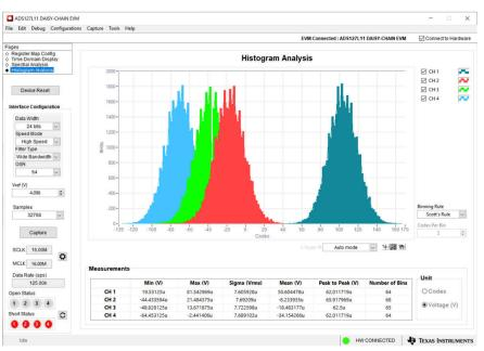
図 4-9. Histogram Plot of ADCs Inputs Shorted (Test Mode)
