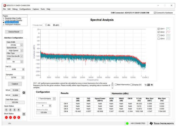
図 4-16. Frequency-Domain Plot of 10-VPP Clock Image Input at Channel 1
