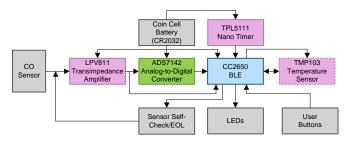
Figure 3. Gas Sensor Node Using ADS7142
