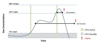
Figure 4. CPU Activity Using the ADS7142
