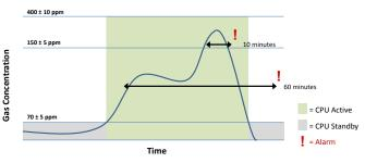
Figure 2. CPU Activity During Non-Alarm Events
