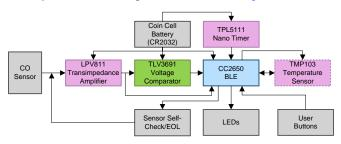
Figure 1. Always-On Gas Sensor Node Design
