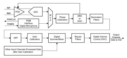
Figure 2-1. AGC Block Diagram
