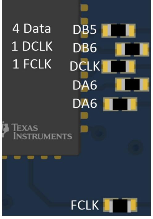
Figure 2-5. ADC3643 Serial CMOS: 2 Wire Resistors
