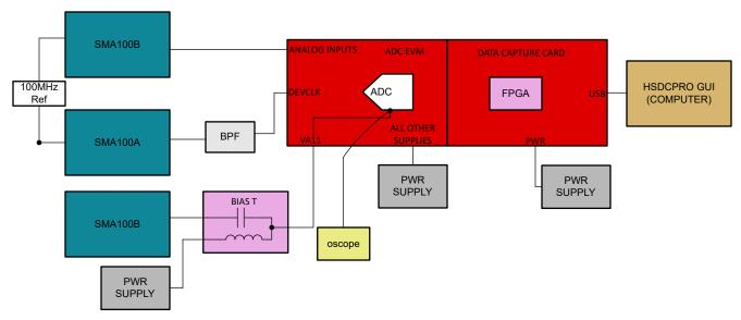
Figure 2-1. Test Configuration for PSRR and PSMR Measurement
