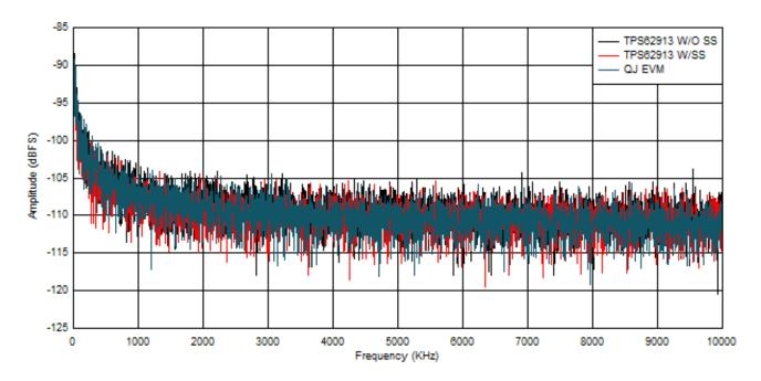
Figure 2-9. PSMR Comparison of Original and TPS62913 at DC
