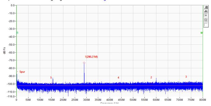
Figure 2-2. Example of Power Supply Rejection Ratio With Forced Error Signal
