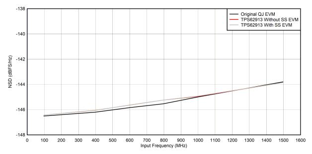
Figure 2-7. Noise Spectral Density Comparison Graph
