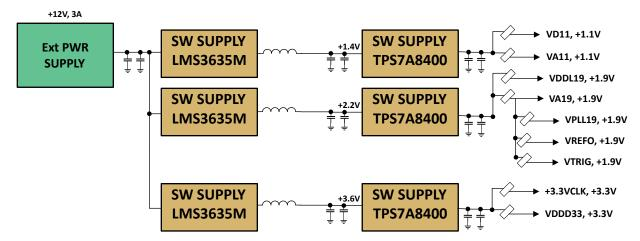
Figure 1-4. Original Power Block Diagram for ADC12QJ1600-Q1 Rev A Evaluation Module
