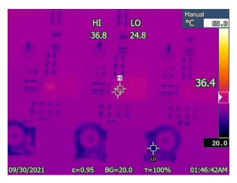
Figure 2-12. TPS62913 Switching Converters
