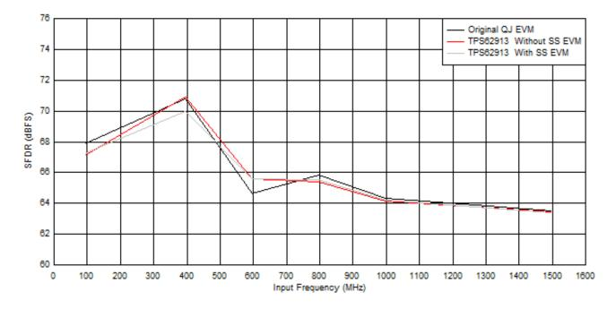
Figure 2-6. Spurious-Free Dynamic Range Comparison Graph
