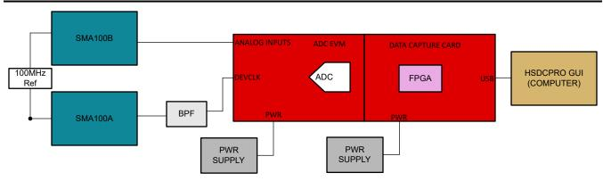
Figure 2-4. Test Configuration for SNR, SFDR, HD, and NSD Measurement
