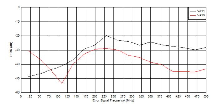
Figure 1-2. ADC12QJ1600-Q1 PSRR of the VA11 and VA19 Supplies
