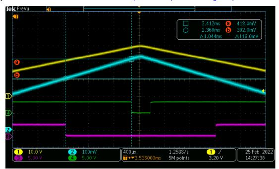
Waveform of IN When V<sub>supp</sub> is Increasing
