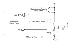
Figure 3. PA Biasing and Current Sensing
