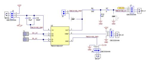
Figure 3-2. TMCS1100 Current-Sensing Circuit
