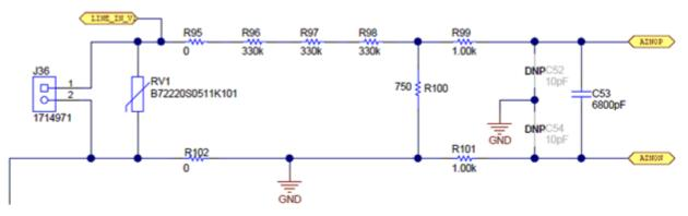
Figure 3-1. Analog Front End for Voltage Inputs
