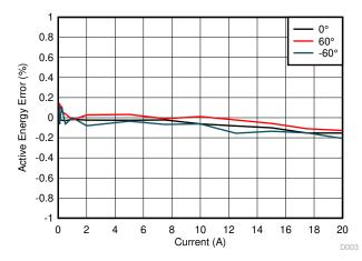
Figure 5-3. Voltage-Current C Mapping Active Energy % Error vs Current
