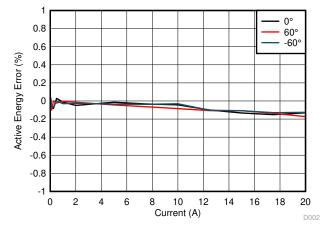
Figure 5-2. Voltage-Current B Mapping Active Energy % Error vs Current
