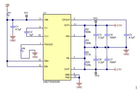
Figure 3-3. TMCS1100 GND and VS Voltage Generation Circuit
