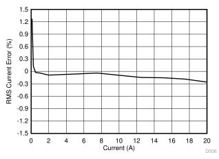
Figure 5-6. RMS Current C % Error
