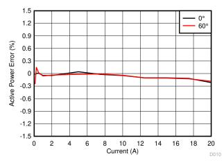
Figure 5-10. Voltage-Current C Mapping Active Power % Error vs Current
