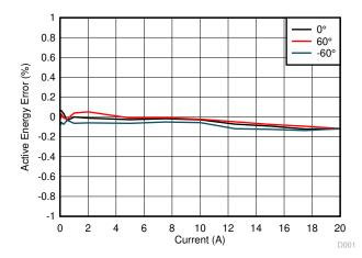
Figure 5-1. Voltage-Current A Mapping Active Energy % Error vs Current
