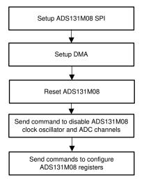
Figure 4-1. ADC Initialization and Synchronization Process
