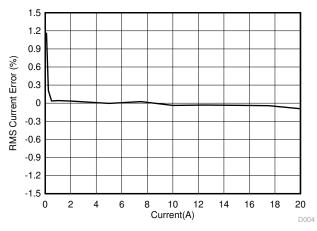
Figure 5-4. RMS Current A % Error
