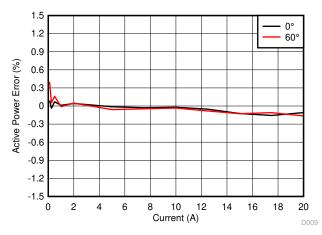
Figure 5-9. Voltage-Current B Mapping Active Power % Error vs Current
