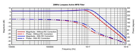
Figure 4. 20MHz Low-Pass Active MFB Filter
