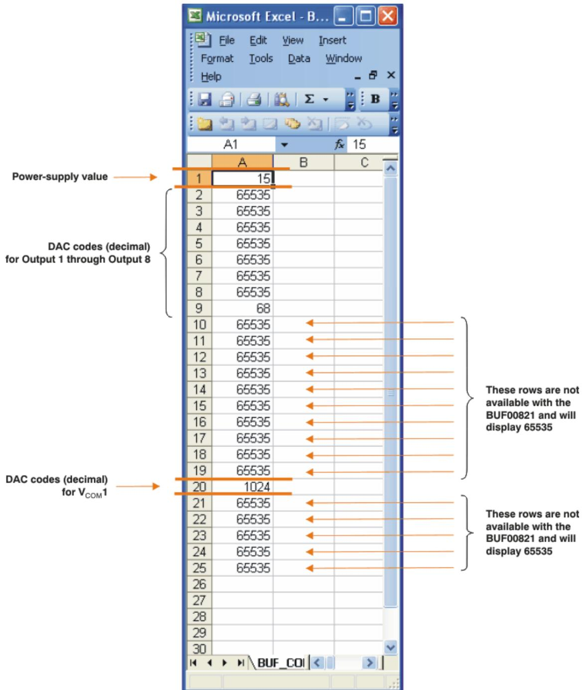
Figure 14. Working with a Saved BUF08821 Data File
