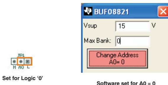
**Figure 7. BUF08821EVM Jumper JP1 Set for Logic '0'**
