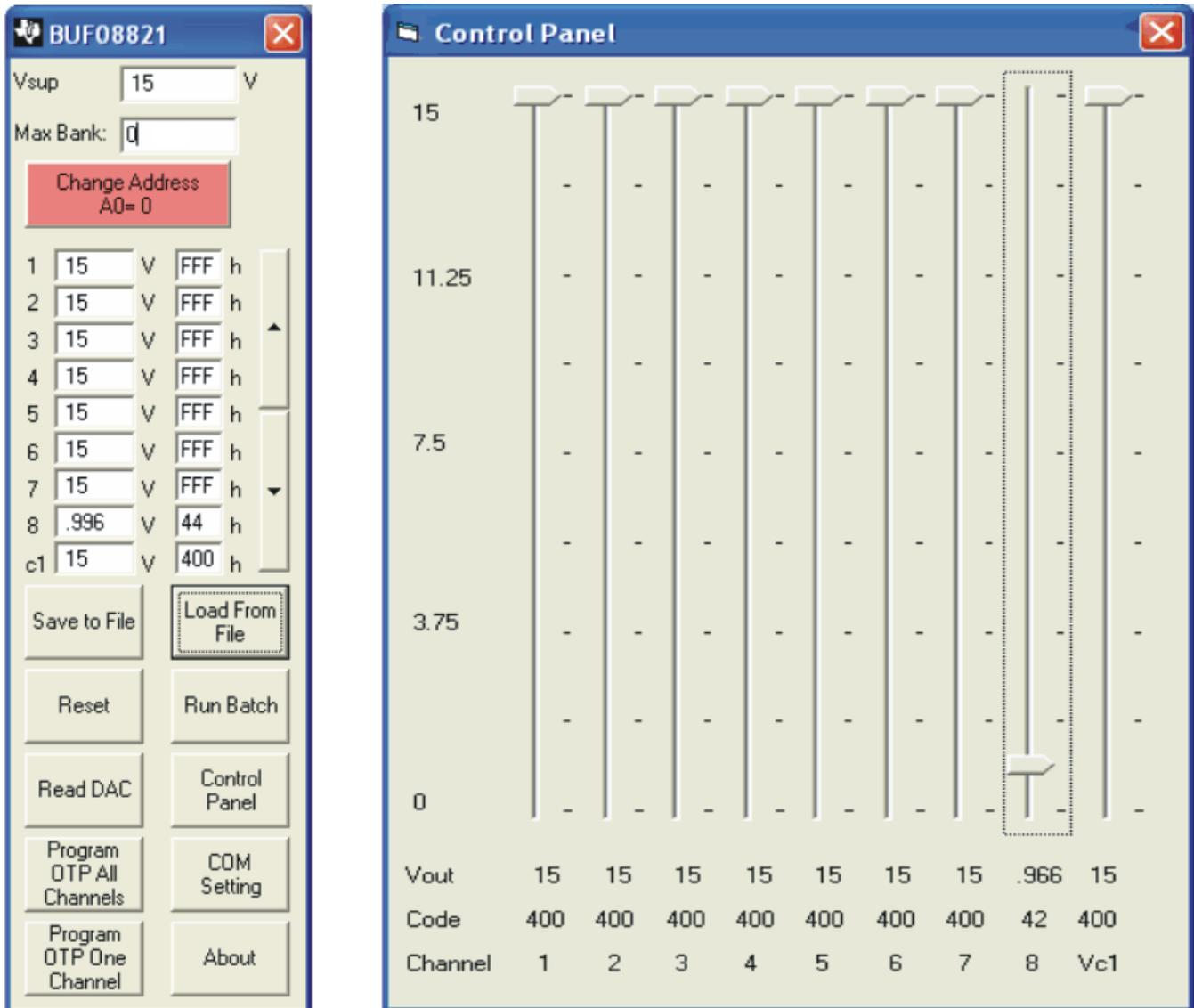
Figure 18. Control Panel Button and Graphical Sliders
