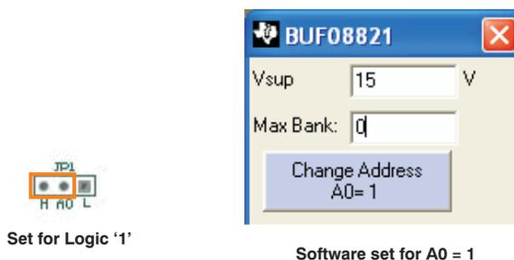
**Figure 6. BUF08821EVM Jumper JP1 Set for Logic '1'**
