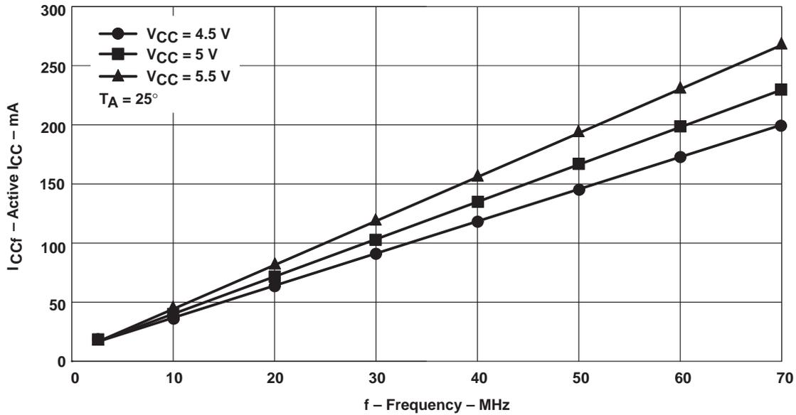
**Figure 4. SN74ACT3632 Active  $I_{CC}$  Versus Frequency**
