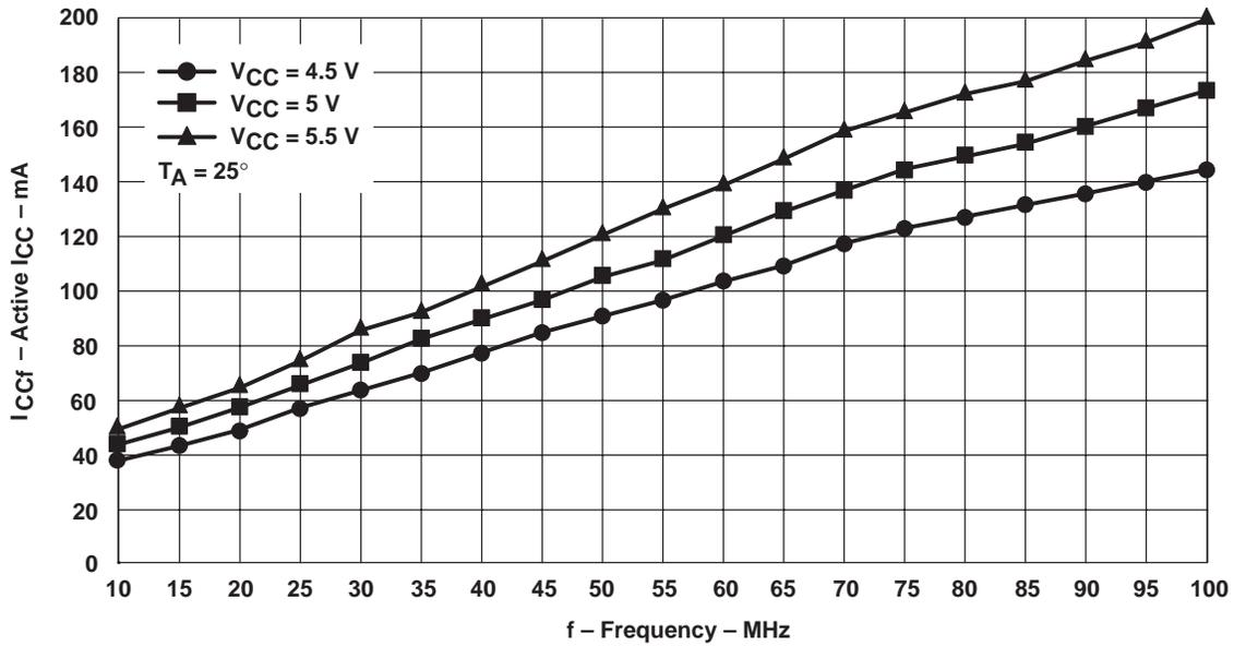
Figure A-9. SN74ABT7819 Active  $I_{CC}$  Versus Frequency
