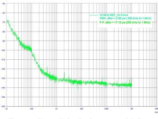
Figure 3. Phase Noise Performance of Agilent E8257C 10MHz REF\_IN
