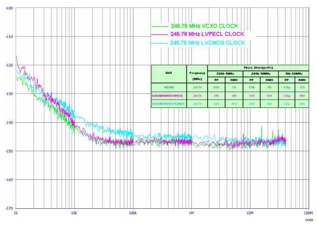
Figure 10. Phase Noise Performance of CDCM7005 Outputs at 245.76 MHz
