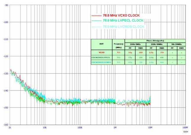
Figure 6. Phase Noise Performance of CDCM7005 Outputs at 76.80 MHz
