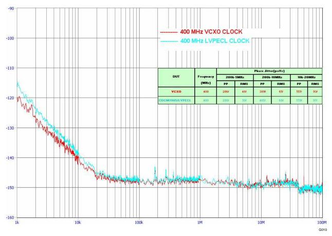
Figure 12. Phase Noise Performance of CDCM7005 Outputs at 400 MHz
