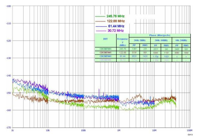
Figure 15. Additive Phase Noise Performance of CDCM7005 LVPECL Output at 245.76 MHz (Buffer Mode)
