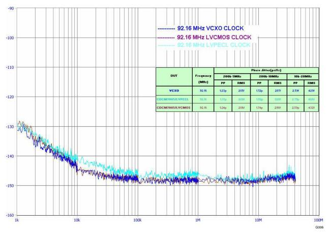
Figure 8. Phase Noise Performance of CDCM7005 Outputs at 92.160 MHz
