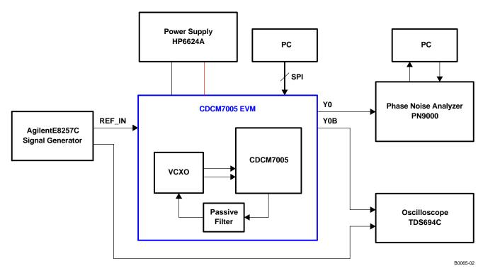
Figure 1. Test Equipment Setup
