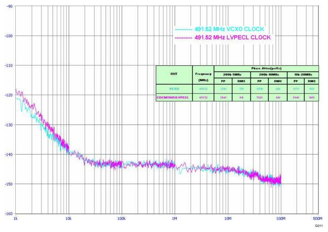
Figure 13. Phase Noise Performance of CDCM7005 Outputs at 491.52 MHz
