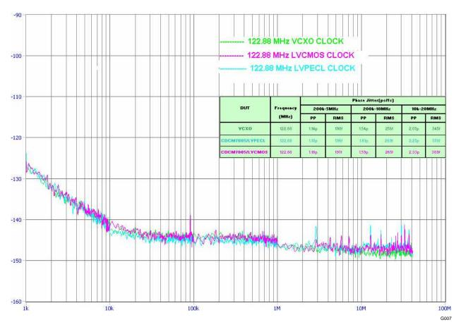
Figure 9. Phase Noise Performance of CDCM7005 Outputs at 122.88 MHz
