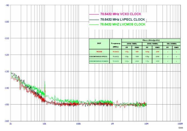
Figure 7. Phase Noise Performance of CDCM7005 Outputs at 78.6432 MHz
