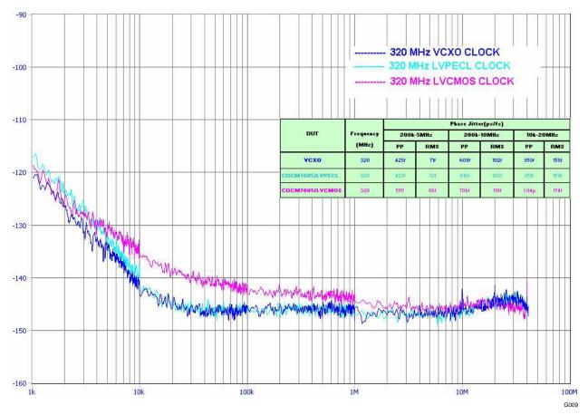
Figure 11. Phase Noise Performance of CDCM7005 Outputs at 320 MHz
