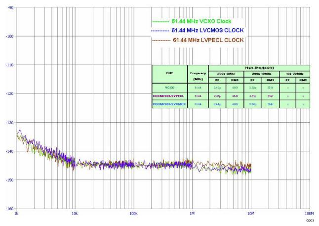
Figure 5. Phase Noise Performance of CDCM7005 Outputs at 61.44 MHz
