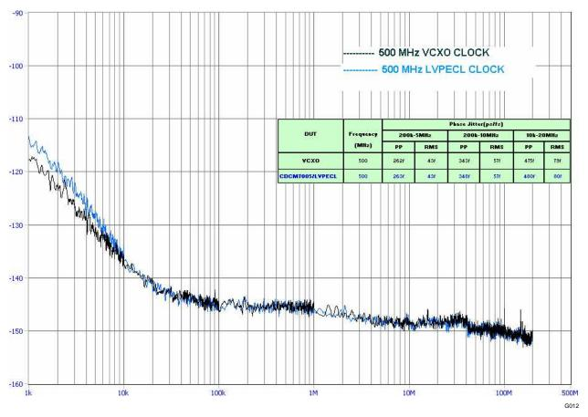
Figure 14. Phase Noise Performance of CDCM7005 Outputs at 500 MHz
