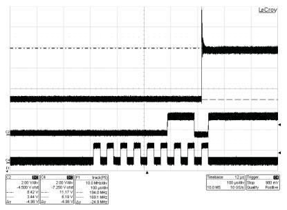
C2 is I2C\_SDA, C4 is I2C\_SCK, and F1 is the frequency on Y1. When byte FS1 (address 13h) is written to 3xh, PLL1 active setup changes from PLL\_setup0 to PLL\_setup1. In this plot, PLL\_setup0 Y1's frequency is set to 170 MHz, and PLL\_setup1 Y1's frequency is set to 194 MHz.
