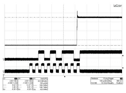
Step 2 to change from 194 MHz to 170 MHz. I2C writeByte 2bxh on address 1bxh (cr(1bxh)=2bxh); the previous contents on that address was cfxh. The change is effective when the last bit on the address 1bxh is patterned. C2 is I2C\_SDA, C4 is I2C\_SCK, and F1 is the frequency on Y1.
