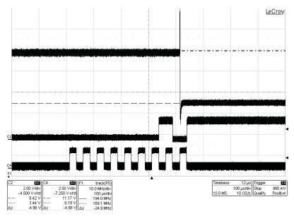
C2 is I2C\_SDA, C4 is I2C\_SCK, and F1 is the frequency on Y1. When byte FS1 (address 13h) is written to 1xh, PLL1 active setup changes from PLL\_setup1 to PLL\_setup0. In this plot, PLL\_setup0 Y1's frequency is set to 170 MHz, and PLL\_setup1 Y1's frequency is set to 194 MHz.
