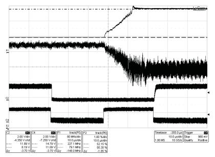
C2 is I2C\_SDA, C4 is I2C\_SCK, F1 is the Y1 frequency, and F2 is Y1 duty cycle. When byte FS1 (address 13h) is written to 03xh, the PLL1 active setup changes from PLL\_setup1 to PLL\_setup0. In this plot, the PLL\_setup0 Y1's frequency is set to 80 MHz, and the PLL\_setup1 Y1's frequency is set to 230 MHz.
