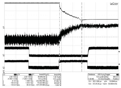
C2 is I2C\_SDA, C4 is I2C\_SCK, F1 is Y1's frequency and F2 is Y1's duty cycle. When byte FS1 (address 13h) is written to 01xh, PLL1 active setup changes from PLL\_setup1 to PLL\_setup0. In this plot, PLL\_setup0 Y1's frequency is set to 230 MHz and PLL\_setup1 Y1's frequency is set to 80 MHz.
