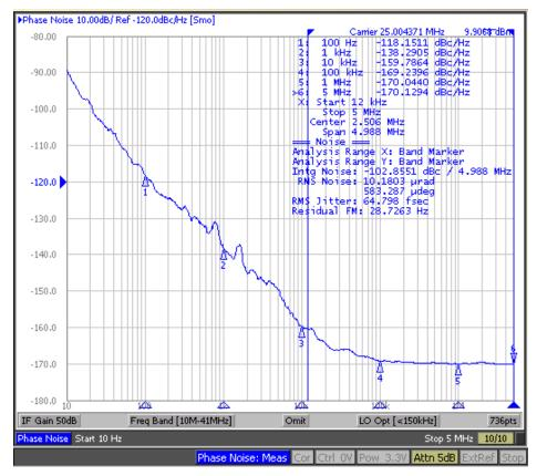
Figure 9. 25-MHz Xtal Output Phase Noise at  $V_{DD} = V_{DDO} = 3.3 V$
