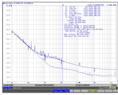
Figure 6. Phase Noise: 80-MHz OCXO (24.9 fs, Light Blue) and Output (83.2 fs, Dark Blue)
