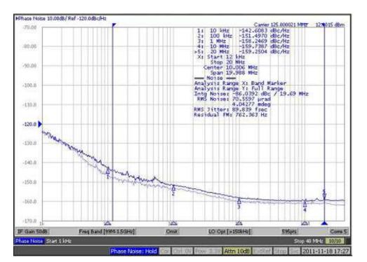
Figure 5. Input Phase Noise (73 fs, Light Blue) and Output Phase Noise (89.8 fs, Dark Blue)
