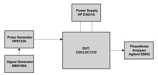
Figure 1. Test Setup for System-Level Additive Jitter Measurements
