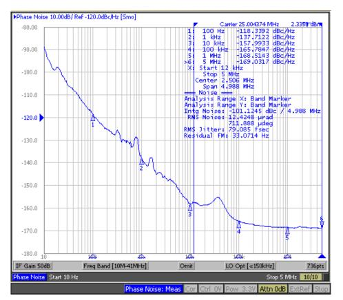
Figure 10. 25-MHz Xtal Output Phase Noise at  $V_{DD}$  = 3.3 V,  $V_{DDO}$  = 1.5 V
