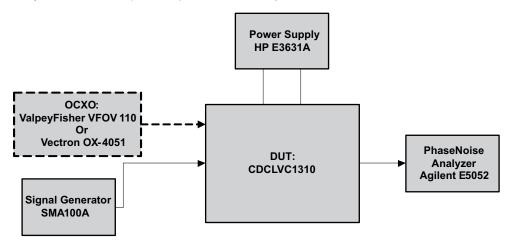
Figure 2. Test Setup for Additive Jitter Measurements
