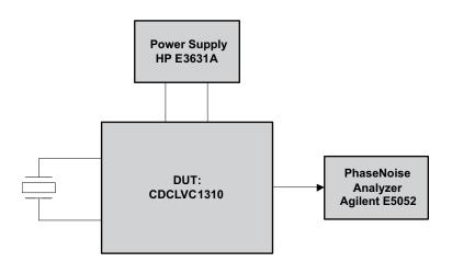
Figure 3. Test Setup for Crystal Oscillator Phase-Noise Measurements
