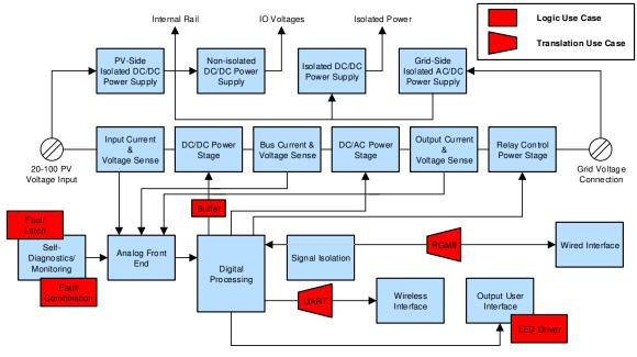
Figure 1. Simplified Block Diagram for Micro Inverters
