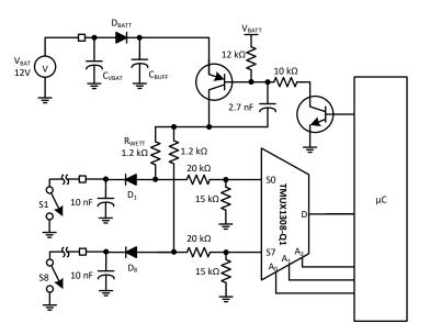
Figure 2-2. Detailed BCM Application with TMUX1308-Q1
