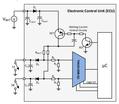
Figure 2-1. Multiplexing BCM Inputs with TMUX1308-Q1
