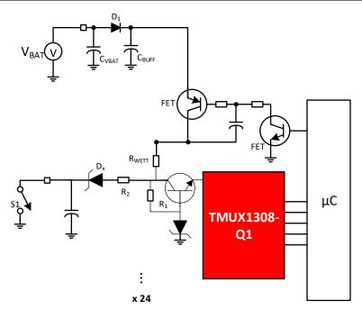
Figure 2-3. 7. Detailed BCM Application with TMUX1308-Q1 and BJT
