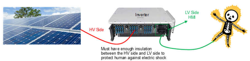
Figure 3-1. Solar Inverter Application Example
