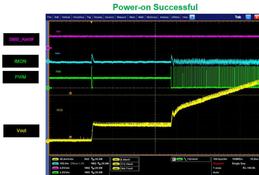
Figure 6-2. Bump Reduction Enable and Final INT_LOW_TC = 1000ns
