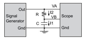
Figure 2. Resistance-capacitor circuit.
