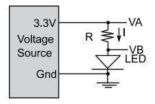
Figure 3. LED test circuit.
