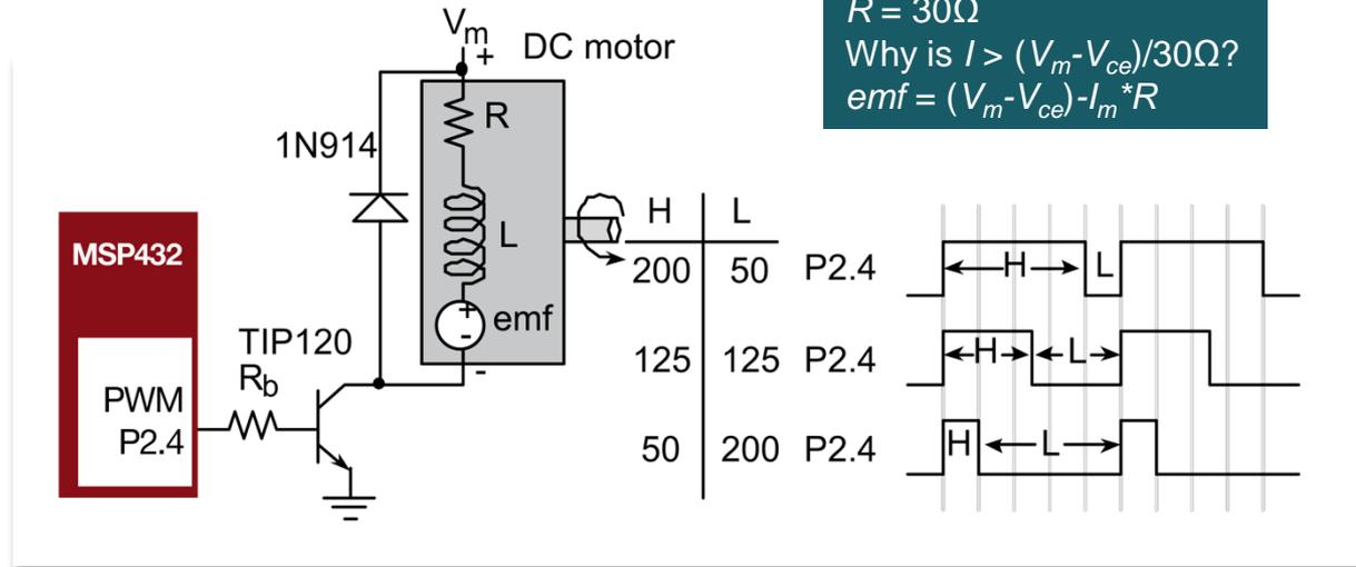
*One direction, power adjusted by duty cycle*
