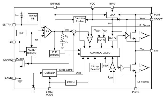
Figure 1-1. Functional Block Diagram
