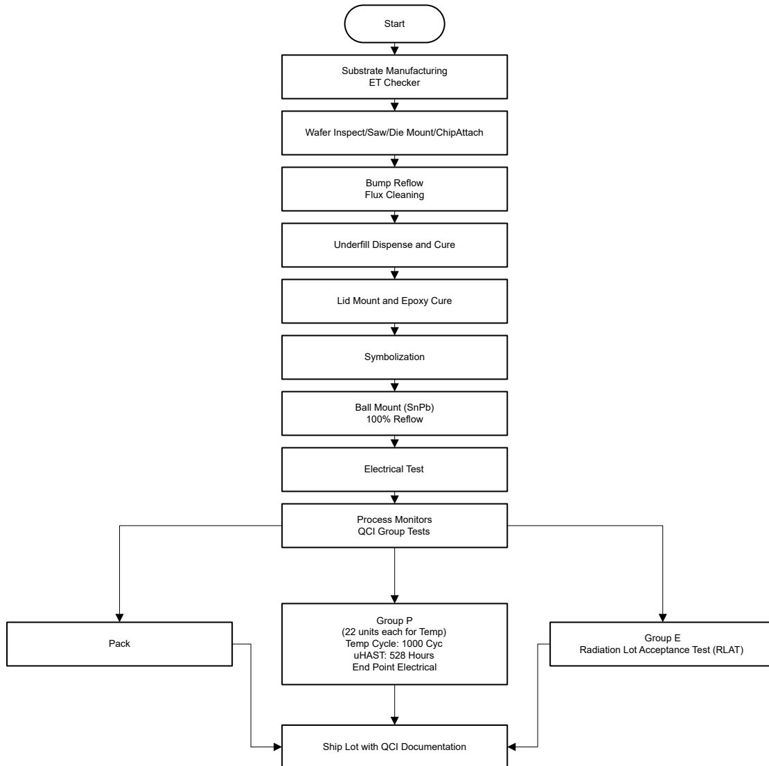
Figure 1-1. AFE7950-SEP Space Enhanced Plastic Production Flow Chart
