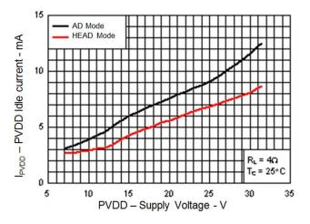
Figure 6. HEAD and AD Idle Current in BTL
