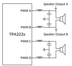
Figure 1. BTL Output Configuration
