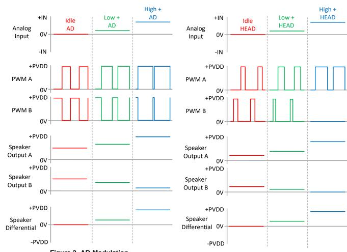
Figure 3. AD Modulation
