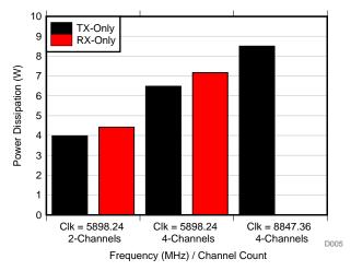
Figure 4. Power Dissipation in TDD Mode
