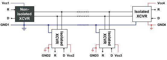
Figure 12. Isolation of Multiple Fieldbus Transceiver Stations
