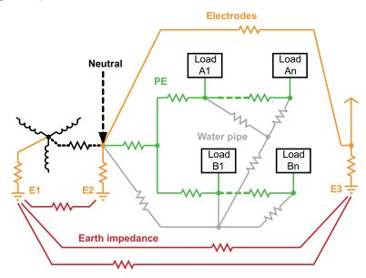
Figure 2. Complex Impedance Model of a Grounding Network
