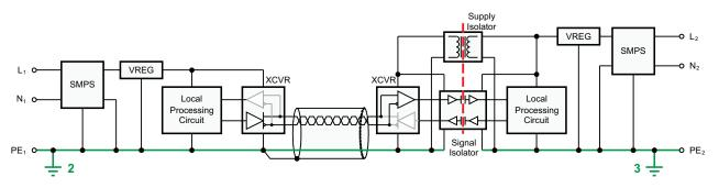
Figure 11. Isolation of Two Remote Transceiver Stations With Single-Ground Reference
