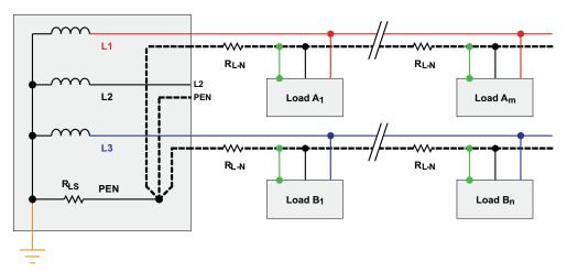
Figure 8. TN-C: The PEN Splits Into Separate Neutral and PE Close to the Loads
