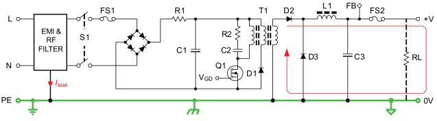
Figure 3. Simplified Block Diagram of an SMPS
