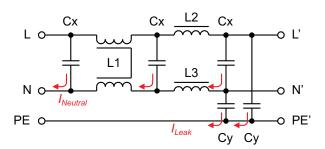
Figure 7. Typical Design of a Single-Phase, Two-Stage EMI Filter
