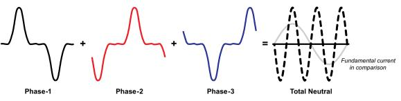
Figure 6. Total Neutral Current Mainly Consists of Third Harmonics
