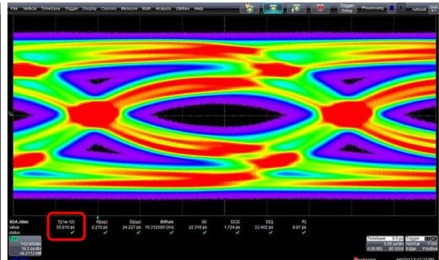
Figure 18. 4" x 4mil Channel – Equalizer Present (Eq=0/-3.5dB Loss)
