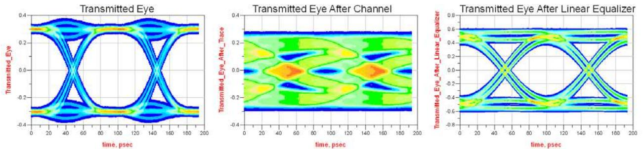
**Figure 12. Eye Diagram - 16in x 4mil Trace**
