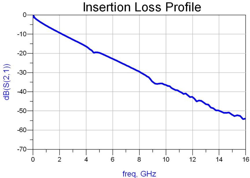
Figure 1. Insertion Loss (SDD21) – 24in x 4mil Trace
