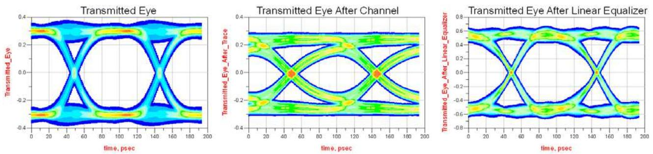
**Figure 10. Eye Diagram - 4in x 4mil Trace**
