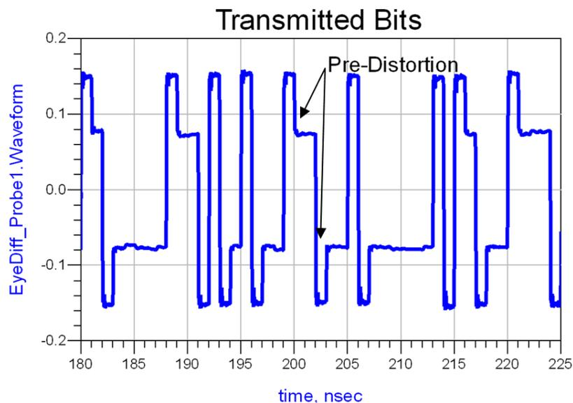
**Figure 3. Transmit Equalization**
