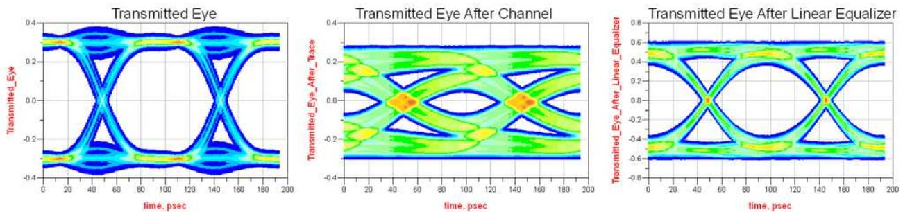
**Figure 11. Eye Diagram - 8in x 4mil Trace**
