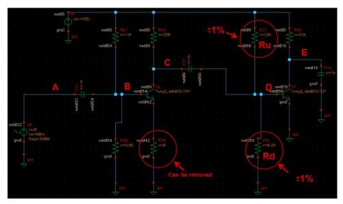
Figure 6. Q-Signal Boost Circuitry for Simulation
