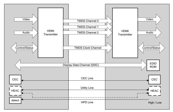
Figure 1. HDMI High-Level Block Diagram
