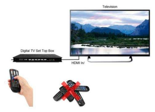
Figure 8. Single Remote Controller for Both HDMI Sink and Source
