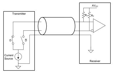
Figure 2. Conceptional Schematic for one TMDS Differential Pair
